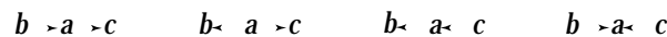
Figure 1.1. Four acyclic digraphs with the vertex set V \equiv \{a, b, c\} . The first three graphs are Markov equivalent: each specifies the single conditional independence X_b \perp X_c | X_a abbreviated as b \perp c | a , while the joint pdf factors as f(a, b, c) = f(b)f(a | b)f(c | a) \equiv f(b | a)f(a)f(c | a) \equiv f(b | a)f(a | c)f(c) . The fourth graph specifies the independence b \perp c and the factorization f(b)f(a | b, c)f(c) .
