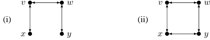
Figure 4: Induced subgraphs of a bi-directed graph with non-orientable edge between v and w .
