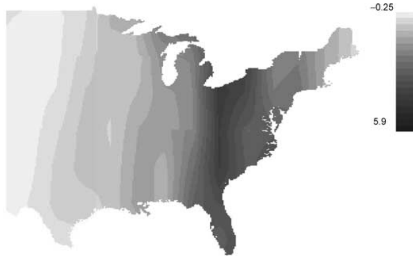
Figure 3. Map of the estimated additive spatial bias of Models-3. The bias parameters are estimated by the means of their posterior distributions.
